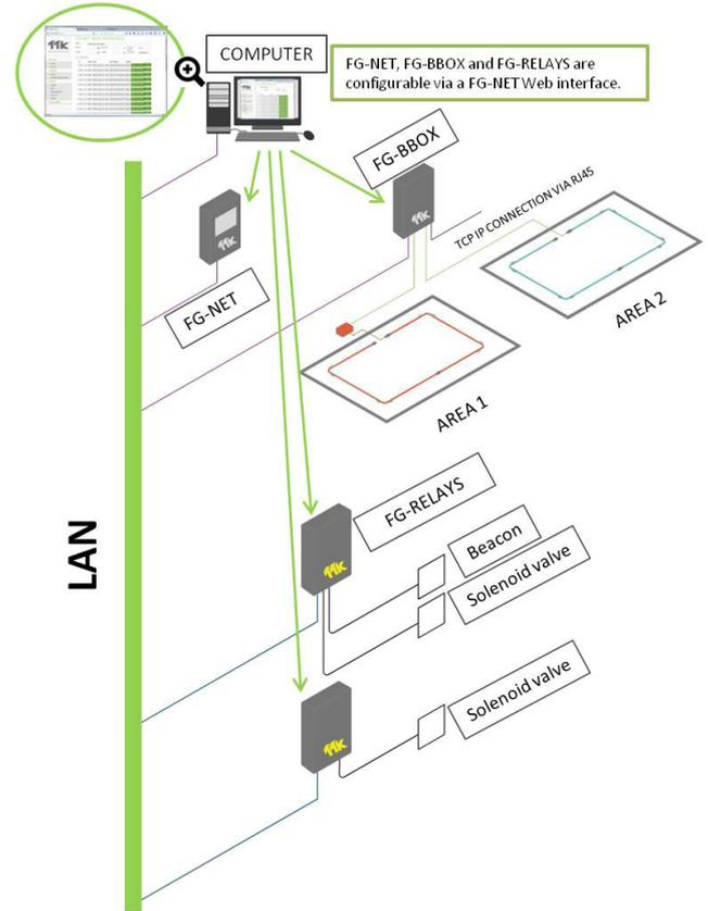
Connection diagram of FG-NET, FG-BBOX, FG-RELAYS and a PC in a Network
