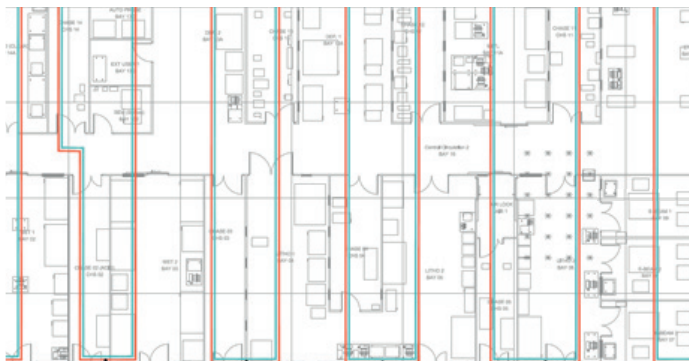
An extract of TTK drawing of hydrocarbon and acid leak detection cables under the raised floor of the laboratory
