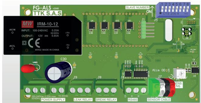
Connect the various cables (leader cable, power supply and relays) at the corresponding connector block.
